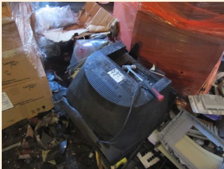
An area inside Sarah's Trading where the manual smashing of Diversified's CRT monitors was taking place. Leaded glass and debris litter the floor. © BAN 2014.
